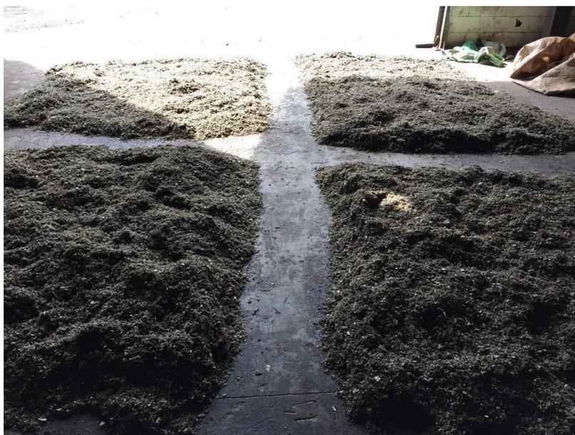
Figura 3.7 – Quarteamento da amostra (FURNAS; CARBOGAS, 2016)
